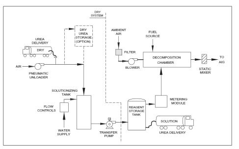
control urea decomposition in a specified temperature window (600-1000 °F). The NOxOUT<sup>®</sup> ULTRA<sup>™</sup> system is simple, consisting of a blower, decomposition chamber, chemical pumping system, urea storage, and process controls.
